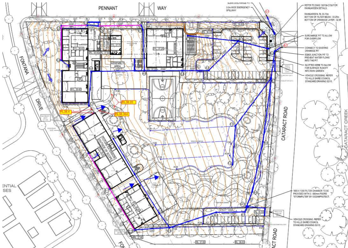
Figure 7. Stormwater System for Proposed Development
