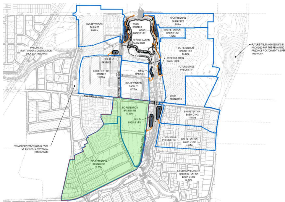
Figure 6. Overall Bio Retention Basins Catchment 200031-LH-DA-C01.51 Rev.3 by Ensipre Solutions
