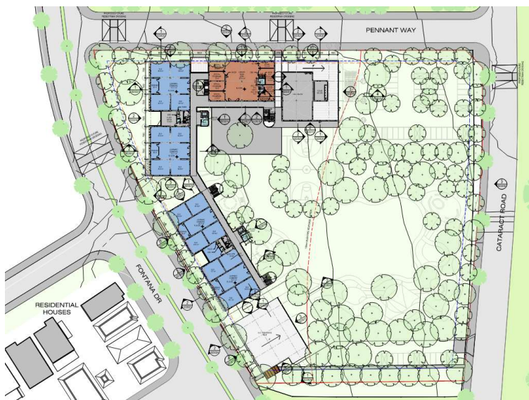
Figure 3. The total school site of 2.21 hectares includes 0.3781 hectares of building area along the Fontana Drive and Pennant Way frontages. The existing site is composed of 100% pervious area. (Source Architectus architectural set)
